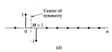
Figure 5.36 Examples of FIR linear-phase systems. (a) Type I, M even, h[n] = h[M - n]. (b) Type II, M odd, h[n] = h[M - n]. (c) Type III, M even, h[n] = -h[M - n]. (d) Type IV, M odd, h[n] = -h[M - n].
